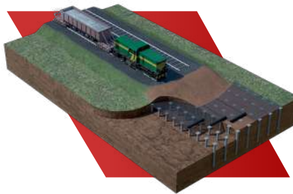
Embankments over rigid inclusions
